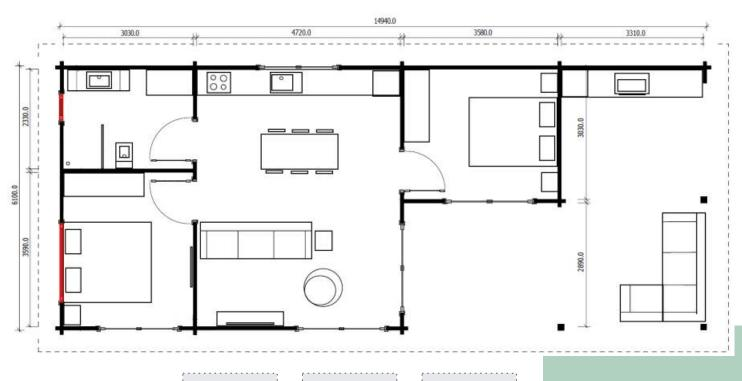
Floor plan wall thickness 80mm which allow to eliminate internal nibs
